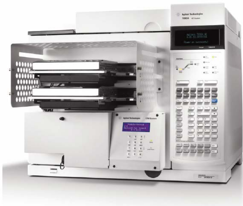
Figure 2. Low thermal mass (LTM) column modules interfaced with the Agilent 7890A GC.
