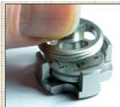
Figure 2. Installing the wafer in the holder
