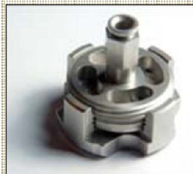
Figure 3. Wafer mounted in the threaded holder
