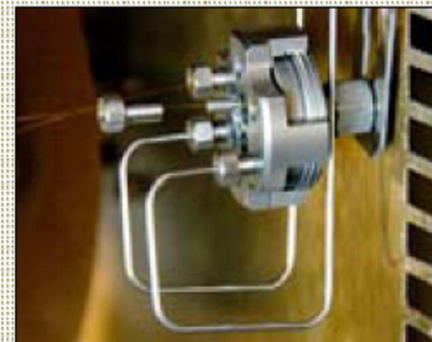
Figure 4. The holder containing the wafer mounted on the GC oven wall and external connections being made.
