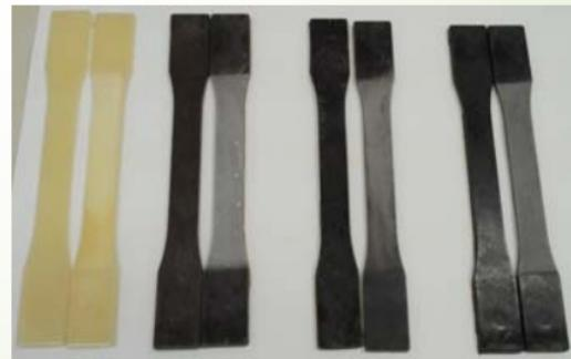
Test samples, before and after aging
